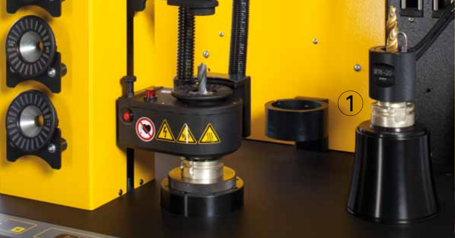
1) Additional holder receptacle Additional mobile receptacle for cooling of holders
